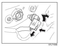
5) Disconnect the coupler with pushing the lock release. Turn the bulb holder counterclockwise and remove it. 6) Replace the bulb, then follow the above steps in reverse to restore the original state.
